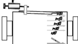
Position 3: Normal house exhaust, grate at midpoint between fully closed and fully open.
