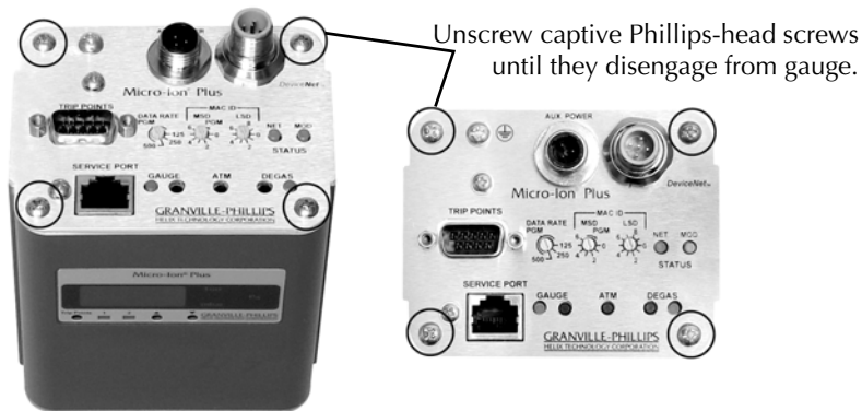
Figure 2 Removing the gauge, Step 3; Replacing the gauge, Step 1
