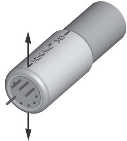
Figure 1 342 or 343 gauge orientation for horizontal mounting
